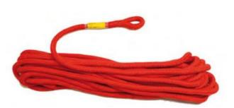
Stranded polyester core with a soft, cotton outersheath. Supplied in 8mm, 10mm, 12mm and 14mm diameters Safe working loads of 127kg,320kg, 400kg, 425kg respectively Factor of safety of 6 to 1 Lengths to suit your requirements. Supplied with spliced eye SWL,Date,Serial No,Length and ID.
